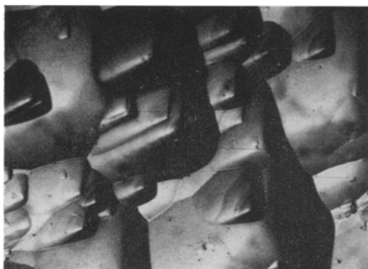
Figure 2 \{111\} surface etched in 1HCl:1HNO 3 for 20 min, showing triangular etch pits ( \times 170 ).
